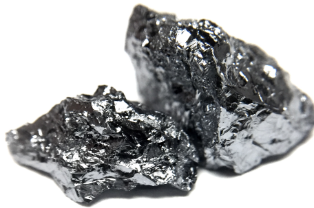
99.9+% Silicon Metal produced by Gen2 during the test #007
