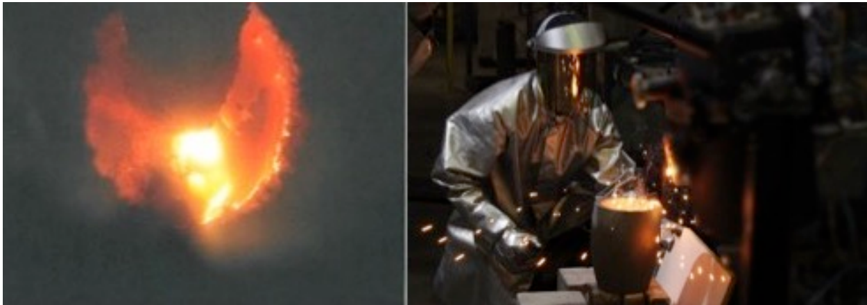
Image 1 compatibility test, left: inside the reactor during the test, right: view of reactor tapping
