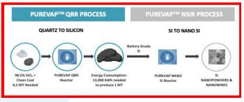
Low-Cost process to transform PUREVAP™ QRR Si into Nano Materials for Batteries
