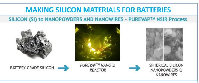
A new scalable, versatile, low-cost plasma process with a capability to produce tailor made spherical Si materials from < 100 nanometer (nm) up to 5 micrometres ( $\mu$ m)
