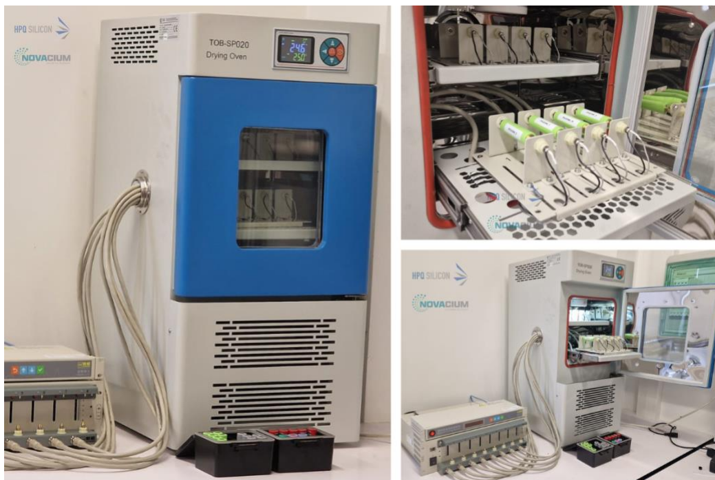
Image collage of the TOB-BTS-5V6A Battery Analyzer. This state-of-the-art 8-channel analyzer, equipped with a climate chamber, enables comprehensive testing of polymer and cylindrical batteries. Key features include precise battery capacity measurement, detailed charge-discharge profiling, and advanced data visualization for accurate performance evaluation.
