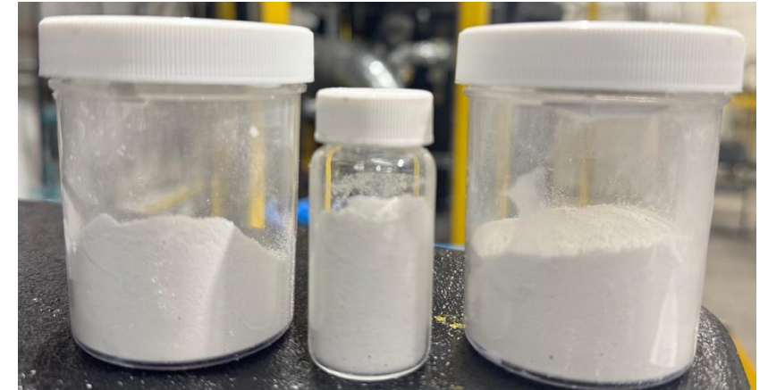
HPQ Fumed Silica produced with Pilot Plant
