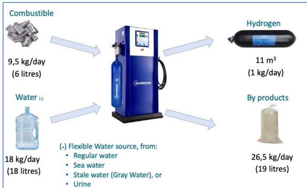
Image 1) Diagram of the METAGENE™ reactor and its green hydrogen production process
