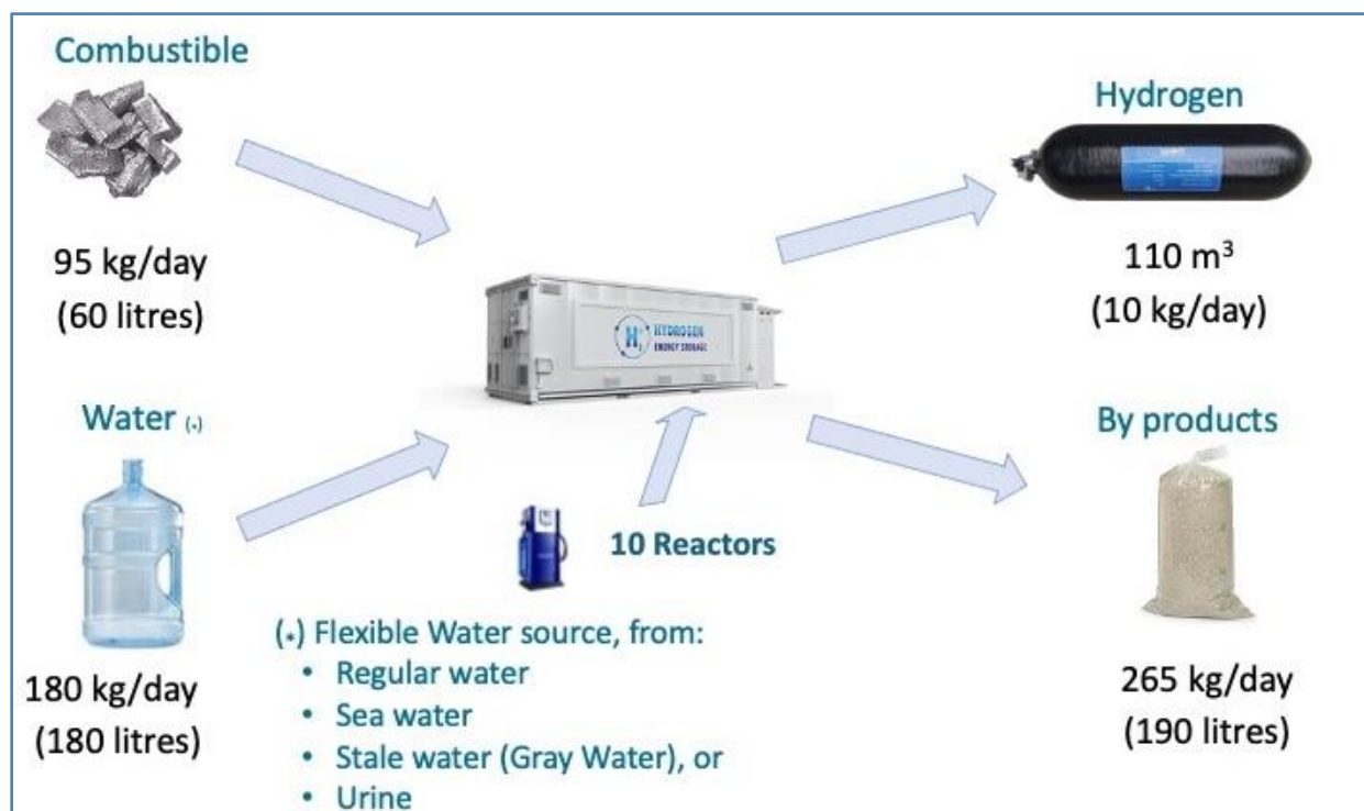
Image 2: Diagram of a METAGENE™ reactor network enabled by the system's flexible and modular design
