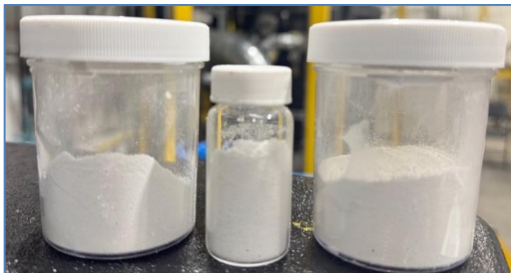
Image 1) Material produced and collected in the baghouse, during the fourth-batch Phase One test, sent to the leading global fumed silica manufacturer under the LOI.
