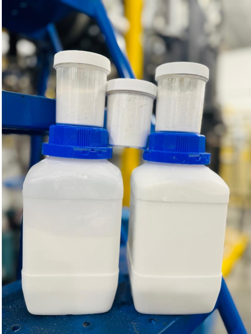
Image 1) Material produced and collected in the baghouse, during Phase 1 Test #5 , and sent to the leading global fumed silica manufacturer under the LOI.
