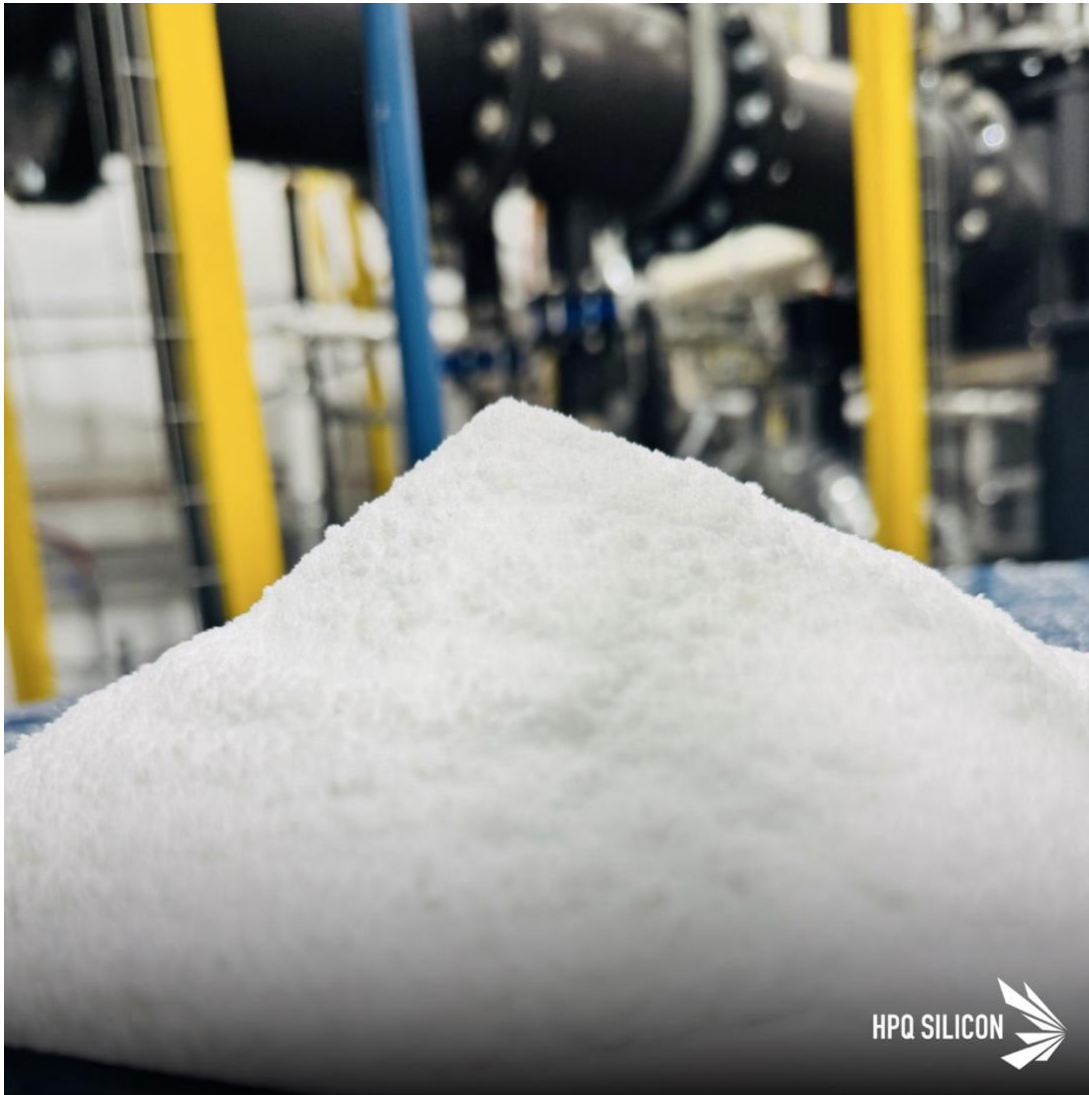
Material produced during test 6 by the Fumed Silica Reactor (Image provided by PyroGenesis).
