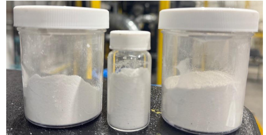
HPQ Fumed Silica produced with Pilot Plant
