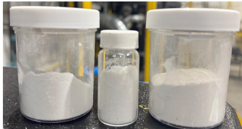
HPQ Fumed Silica produced with Pilot Plant
